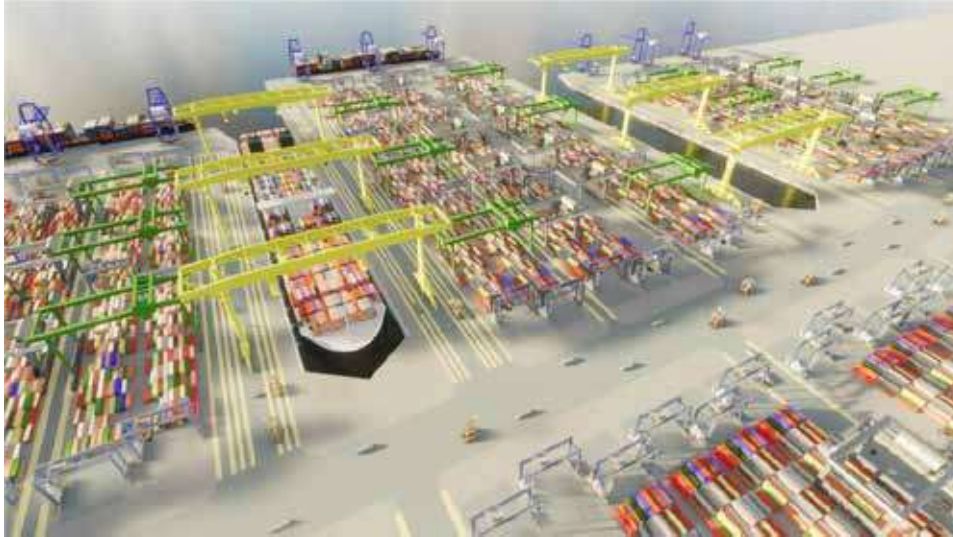
Figure 4: Proposal for a terminal layout with two indented berths.
